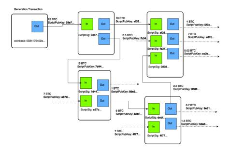
Figure 1: An example of transaction chaining in Bitcoin.
